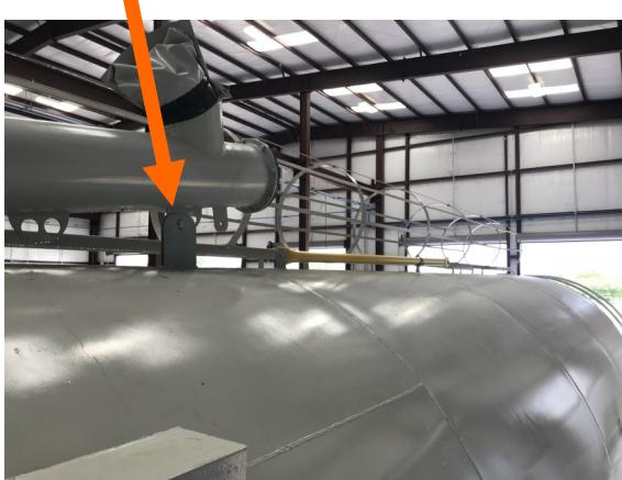
Step Two: Use the hand winch to lower the auger into place. It has a built in break so You just turn the handle to lower or raise.
