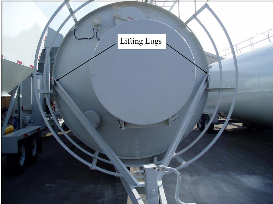
It is best to place the lifting Straps on the outside of the Railing when standing up the silo so as to not damage the hand railings.
