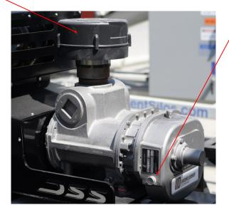
Keep an eye on the blower oil level—The oil should be 1/2 full in the sight glass.
