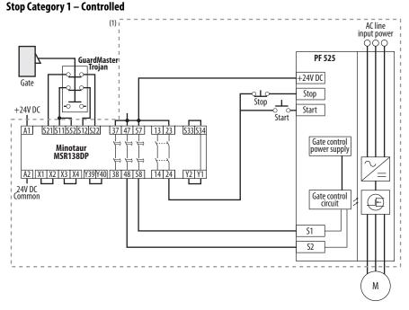
Enclosure Recommended. External wiring failure modes must be considered as described in EN ISO 13849-2. Enclosure or other measure to exclude these failure modes should be used.
