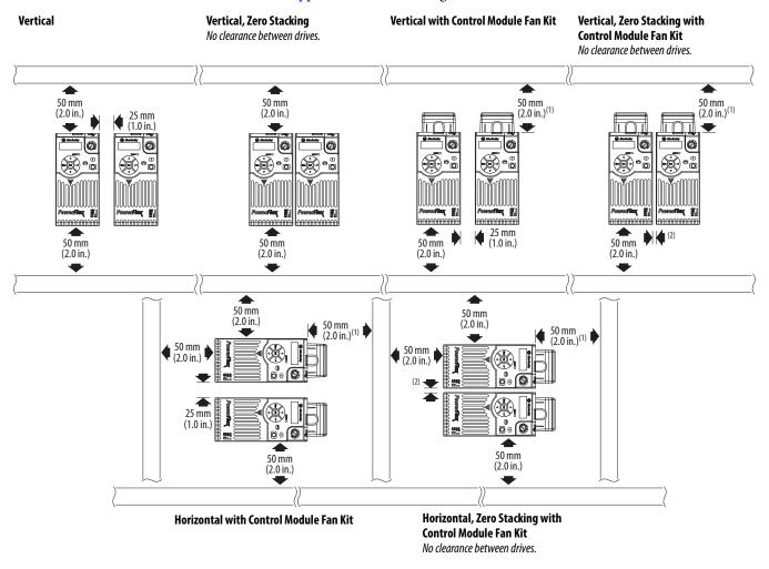
(1) For Frame E with Control Module Fan Kit only, clearance of 95 mm (3.7 in.) is required.
