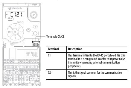
Connect terminal CS1 or CS2 to a clean ground when using a network with a ring topology.
