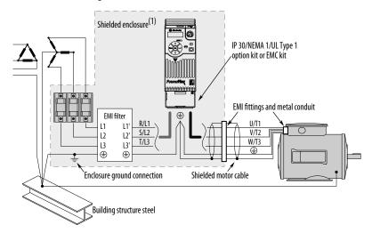
(1) Some installations require a shielded enclosure. Keep wire length as short as possible between the enclosure entry point and the EMI filter.
