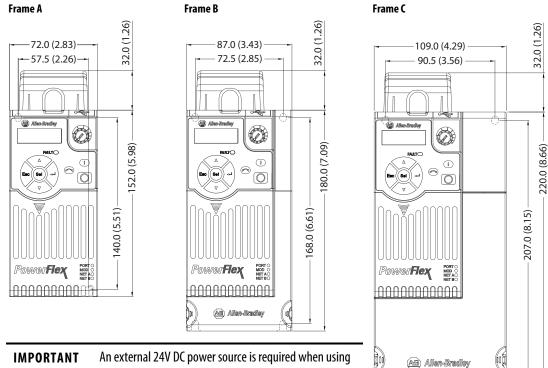
the Control Module Fan Kit with drive frames A, B, and C.
