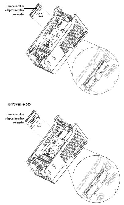
**2.** Align the connectors on the communication adapter to the communication adapter interface connector, then push the back cover down.
