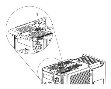
**3.** Hold the sides and top of the Control Module firmly, then pull out to separate it from the Power Module.
