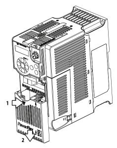
Re-attach the front cover when wiring is complete.
