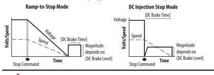
**ATTENTION:** If a hazard of injury due to movement of equipment or material exists, an auxiliary mechanical braking device must be used. This feature should not be used with synchronous motors. Motors may be demagnetized during braking.
