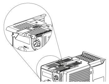
**3.** Insert the catch at the top of the frame cover into the Power Module, then swing the frame cover to snap the side catches onto the Power Module (Frames B...E only).
