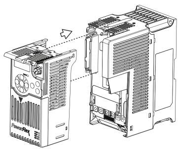
2. Push the top cover of the Control Module towards the Power Module to lock it.
