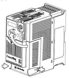
**2.** Press down and slide out the top cover of the Control Module to unlock it from the Power Module.
